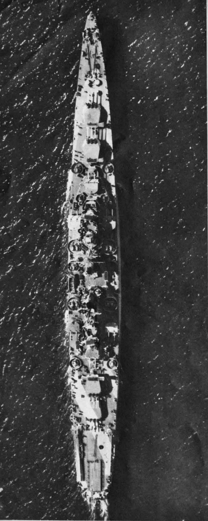
Old cruiser's decks are shorter and less spacious than on new type (left). The sides are shallow curve from pointed bow to tapered stern.
